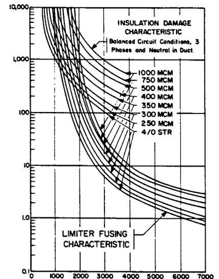
Figure 4: Current - Amperes Standard 250 Volt Limiters
