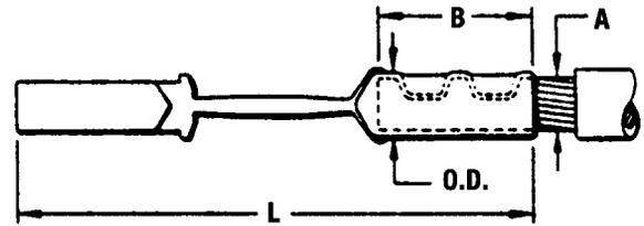
\*Paper Insulated Cable - Oil Tight Cable Sockets.
