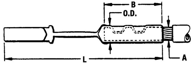
To specify a fast acting limiter in any configuration insert an "F" before the conductor number (e.g., YFSF34CR specifies a 1/2 thick limiter section).
