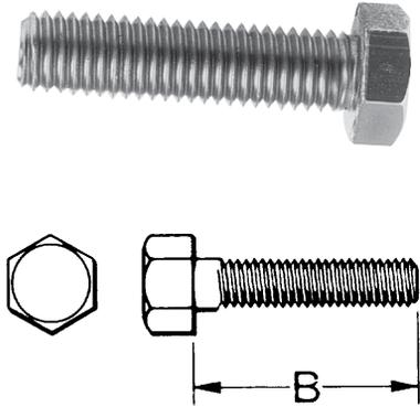
BURNDY® aluminum hexagon head bolts are manufactured of alloy 2024-T4 and are finished with anodic coating and lubricated. Threads are coarse series, class 2A fit.
