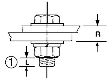
† For use with CUSA750-2TC38 copper spacer adaptor, (2) terminals and " thick equipment bus bar. For other combinations contact BURNDY®.
